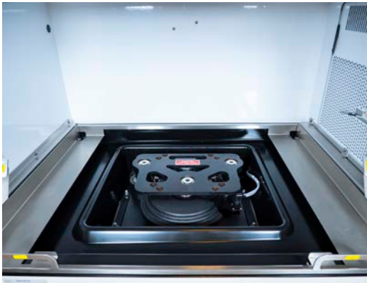
Vibration- and trouble-free operation for years: Three weight-supporting shafts, nine permanently lubricated ball bearings and the large platform bearing surface support the platform load
